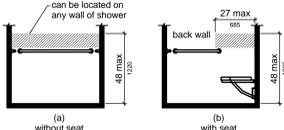
Figure 608.5.2 Standard Roll-in Type Shower Compartment Control
