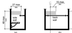
Figure 608.5.3 Alternate Roll-in Type Shower Compartment Control
