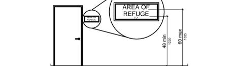
Figure 703.4 Height of Tactile Characters Above Finish Floor or Ground
