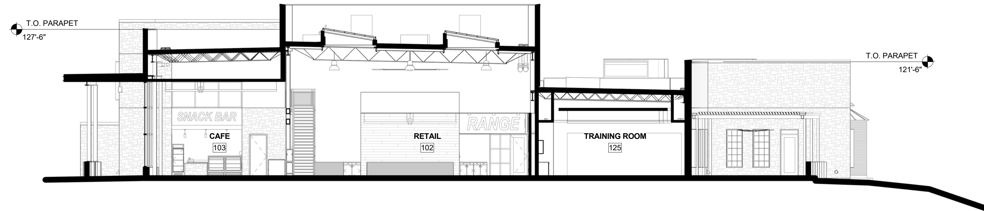
BUILDING SECTION ( NORTH - SOUTH ) 01 | 1 SCALE: 3/32" = 1'-0" A4.12
